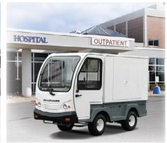
The ET-3000 electric utility vehicle competes with gasoline vehicles in outdoor applications. This vehicle operates at 18 mph and carries loads up to 3,000 lb. Specifically designed to meet rugged outdoor applications, the ET-3000 is equipped with a 48 volt drive train that travels up to 30 miles in a single charge.
