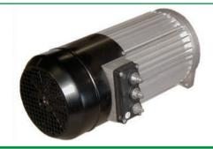
Enclosed "AC" induction 17 HP motor with thermal protection. External "fin" cooling from mechanical driven fan. Includes an automatic parking brake feature.
