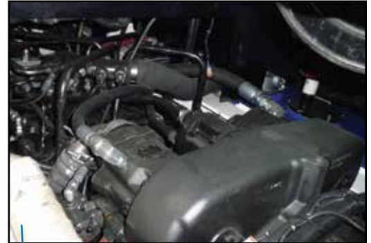
Daily checks and routine maintenance are simple with easy-lift hood, which is supported by a gas cylinder. Once opened, fluid, filter and other service points are immediately within reach.
