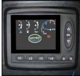
MD3 display provides operator filter restriction alerts.
