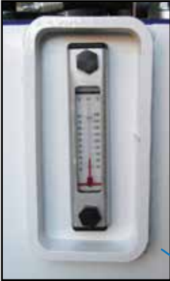
Hydraulic oil level temperature gauge is located on the side of the liftruck for easy viewing.
