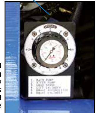
Hydraulic pressure can be easily read by lifting up a flip-open step and twisting gauge. This eliminates downtime due to hydraulic system issues and eliminates the need to tap into hydraulic lines and potentially contaminate the marine environment.
