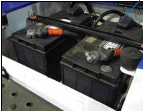
Located on both sides of the forklift, flip-open panels allow quick and easy access to the complete drive line, batteries and hydraulic multi-gauge.
