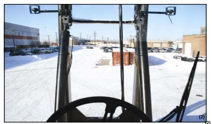
Operator has unobstructed visibility through the mast (above), upward through the angled glass on top of the cab (below). Excellent operator visibility at all load elevations without having to adjust body position.
