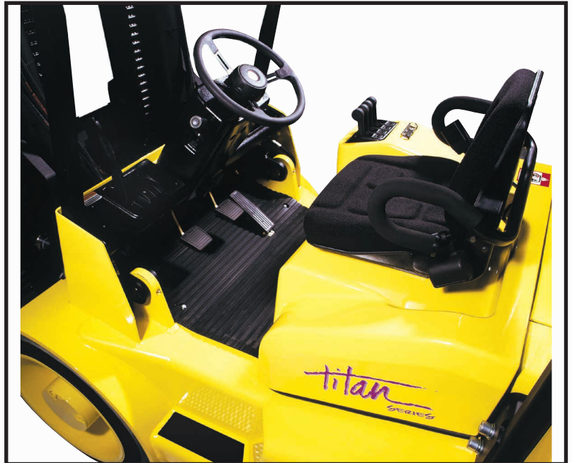
The operator platform meets ANSI B56.1 FOPS operator protection.
