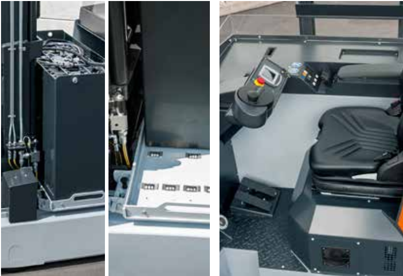
Easy battery exchange via roller table
