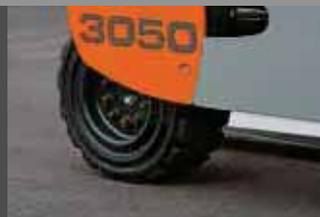
The soft elastic tyres are particularly suitable for poor floor and ground conditions and increase the driving comfort at the same time. Since the hydraulic hoses for the travel motors are located in the load bed, the components are protected against damage.
