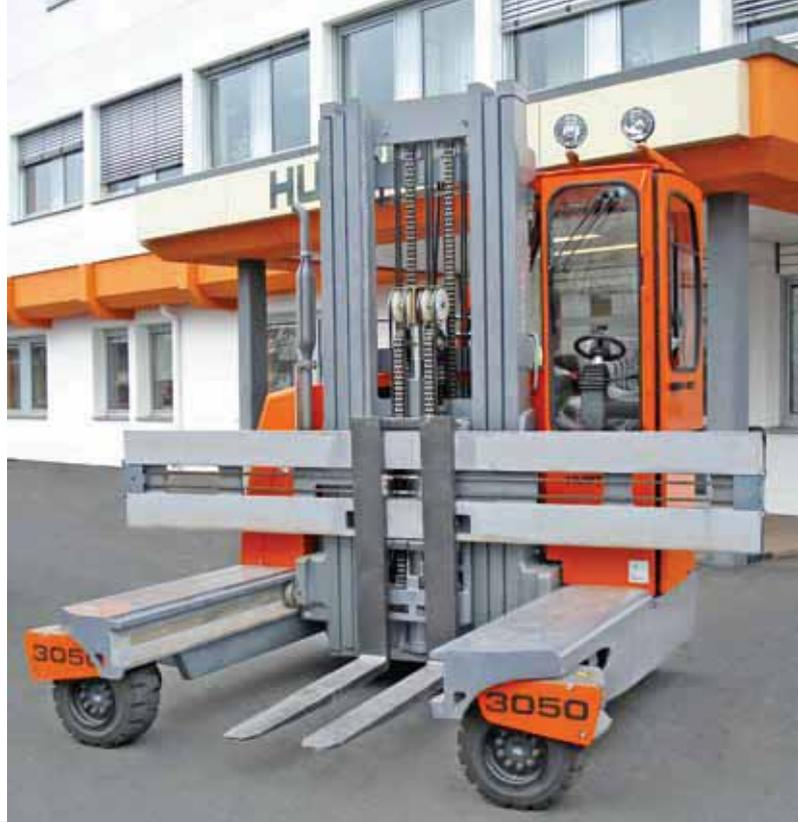
➤ **Two-stage lift mast with full free lift (Duplex)**
