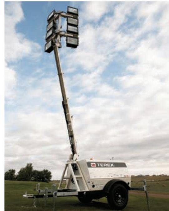
**Brilliant Features: UHMW side pads are incorporated throughout all Terex light tower mast systems to help provide longer mast life, less friction and a higher level of corrosion resistance by eliminating metal-to-metal mast wear.**
