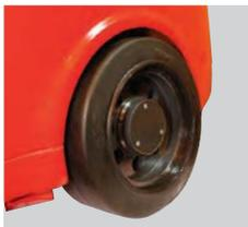
Cushion tires allow operation on standard warehouse floors. Low point loadings compared to guided VNA trucks.
