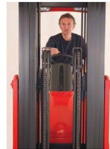
Flexi's famous "clear vision" mast is available in either triplex or quad format. Integrated side shift fork carriage is standard.
