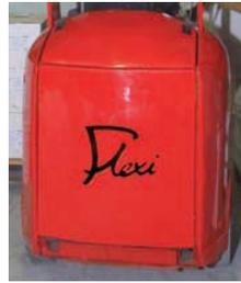
Detailed steel plate rear panel protects traction battery. Narrow 38" wide rear chassis allows block stacking and drive in rack operation.
