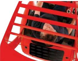
The unique 'Hi Vis' safety guard combines maximum visibility and overhead protection for the operator.
