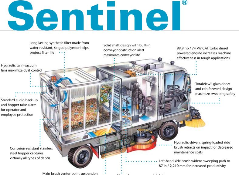
Main brush center-point suspension for sweeping uneven surface types
