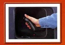
Toyota's intuitively-mapped, multi-functional control handle lets operators simultaneously control travel, lift or lower plus access the horn.
