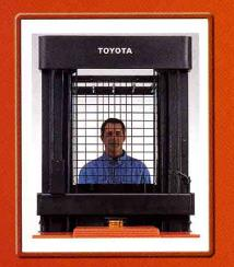
Toyota's wide-view mast with nested mast channels and electronic cushioning helps provide smooth load handling, reduced operator fatigue and even higher levels of productivity.
