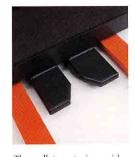
The pallet centering guide with automatic clamp and release foot pedal helps provide convenient and efficient pallet handling.
