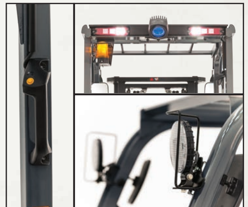
Pictured: Rear assist grip with horn (left), reverse activated blue light (top), front LED combination lights (bottom)
