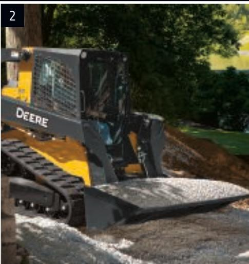
1. Fast ground speeds and large bucket capacities enable these nimble material movers to make the most of every cycle. For even more hustle, engage the two-speed transmission (optional on the 323E; not available on the 319E).
