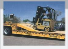
The hydraulic recessed upper deck ramp allows you to load the upper deck and maximize your hauling capacity.
