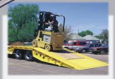
With the push of a lever, the hydraulic tail can be lowered to load from ground level...
