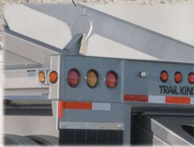
Two-Component Paint Finish The entire trailer is primed and painted with a two-component polyurethane primer and paint, after which electrical lines are installed
