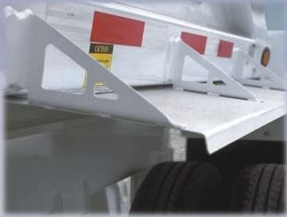
Full-Width Fenders, both front and rear, are sloped to shed material more effectively.
