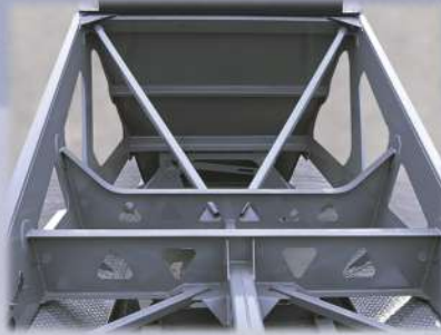
Lightweight Crossbraces tie the frame together in a way that minimizes the flexing and twisting that can cause cracking in critical stress areas.
