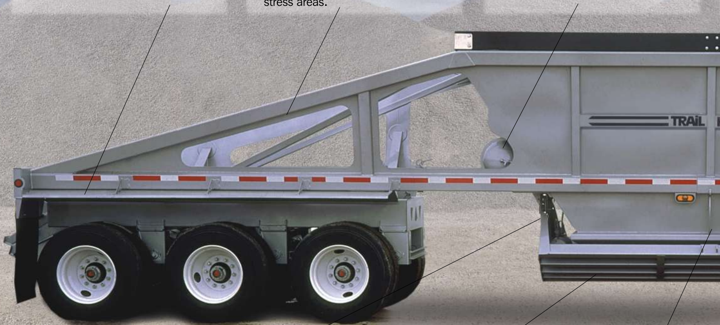
Lightweight Crossbraces tie the frame together in a way that minimizes the flexing and twisting that can cause cracking in critical stress areas.
