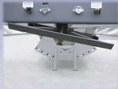
Full Oscillating Fifth Wheel Plate features a spherical, chrome-bushed design that reduces wear and provides longer service life than a shaft and bushing design.
