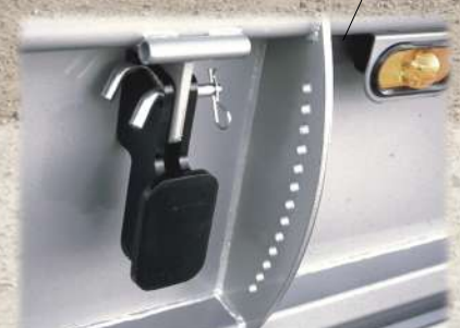
Adjustable 11-Position Gate Stop is conveniently positioned on the side of the hopper so the gate setting can be adjusted without crawling under the trailer.
