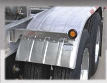
One-piece fender brackets are lightweight, incorporate the LED (standard) lights right into the bracket, and bolt-on for easy maintenance or replacement.
