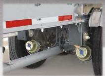
Hendrickson Intraax AANT23K Tapered Beam Suspensions are among the lightest suspensions available and come standard with black undercoating for a long-lasting, chip-resistant finish.
