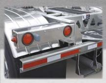
The light box is lightweight, and its bolt-on modular design makes repair or maintenance easier. The beehive-style LED (standard) light on the end of the light box is easier for the operator to view from the cab.
