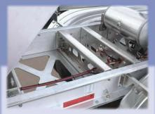
Formed aluminum cross members span the full depth of the end frame and a new, lightweight aluminum torsion plate runs the full width and length of the end frame for maximum structural strength and weight savings.
