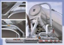
Mandrel bent piping throughout the trailer allows for unobstructed flow of product, thereby reducing heat and friction, and delivering faster, trouble-free unloading.
