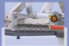
The bolted, adjustable "severe service" upper coupler plate delivers "muscle"... the fender bracket (that doubles a protection for the wiring hamess) and bolt-on hose tube (that makes hanging the hot air hose for transport quick and easy) deliver weight savings.
