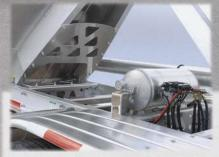
The weight savings of standard components such as the aluminum air tank and the thinner, more streamlined torsion plates make the "1033" incredibly lightweight.
