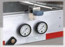
Easy-to-read, liquid-filled gauges are conveniently located on the side of the trailer frame.
