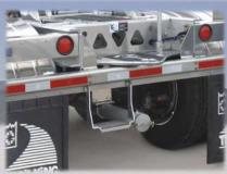
Rear discharge pipe can be positioned in several configurations: under, over or, if an inverted axle is specified, straight through the axle. Lightweight bolt-on modular components, such as the bumper and light boxes, make repair/replacement easy.
