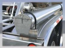
The hose tube is reinforced at both ends to prevent damage from the metal ends of the discharge hose during transport. The hose tube hanger is formed, rather than welded, for a lighter, easier-to-repair/replace design.
