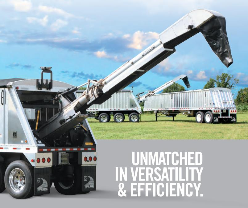
Trail King's Aluminum Grain Hopper Conveyor Trailer is the most advanced and reliable multi-purpose trailer unit in the industry. A strong stainless steel conveyor attaches to our standard aluminum grain hopper trailer with the option to be removable. Designed as light as 13,516 lbs., you will have the freedom to haul more in every load. Faster seeding and fertilizing made possible with hauling capacities of up to 1,402 bushels (heaped).
