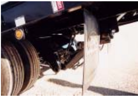
Heavy duty Etnyre folding tail design.
