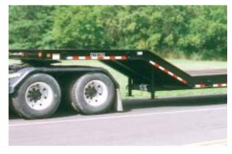
The full width gooseneck with a 3 to 1 slope accommodates most rollers.
