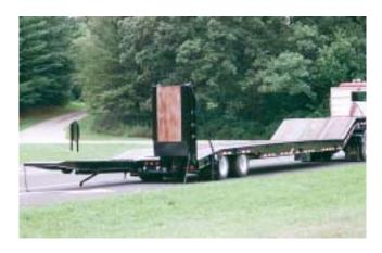
One man operation with electric/hydraulic bifold operated ramps. Shown with optional 12' ramps.
