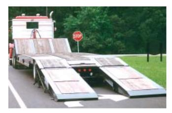
The standard manual exhaust feature on the air suspension enhances the low rear climb angles. Shown with optional 12' ramps.
