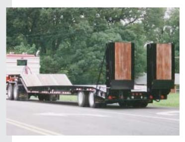
Fast and easy hydraulically operated bi-fold ramps. Shown with optional 12' ramps.
