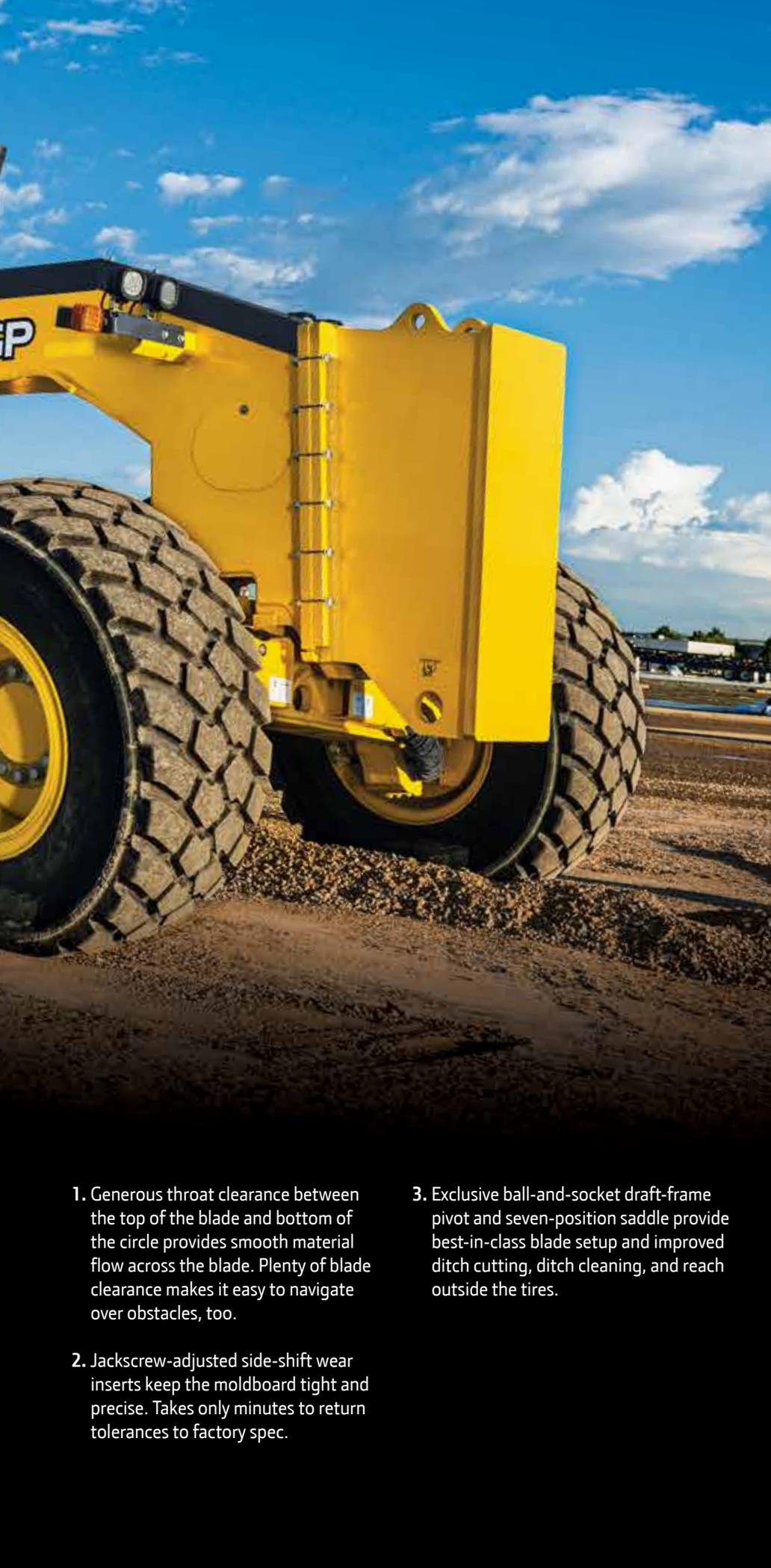
1. Generous throat clearance between the top of the blade and bottom of the circle provides smooth material flow across the blade. Plenty of blade clearance makes it easy to navigate over obstacles, too.
