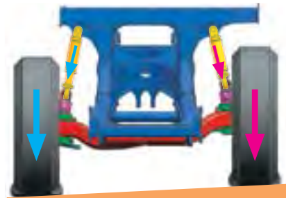
DRIVER SIDE STRUT IN COMPRESSION, OTHER STRUT IN EXTENSION
