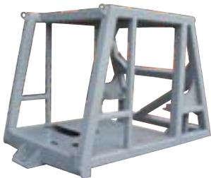
Our new cab structure provides improved safety and durability. The cab frame is stronger and features a three-point isolation-mount design to allow additional independent motion from the truck frame.
