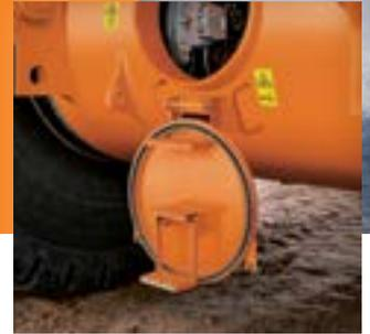
■ The collapsible step and flat service stage inside the rear axle brings higher serviceability and safety.
