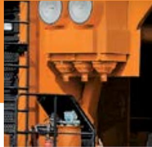
■ Four, low maintenance air filters with evacuator valves bring easy and safe maintenance.
