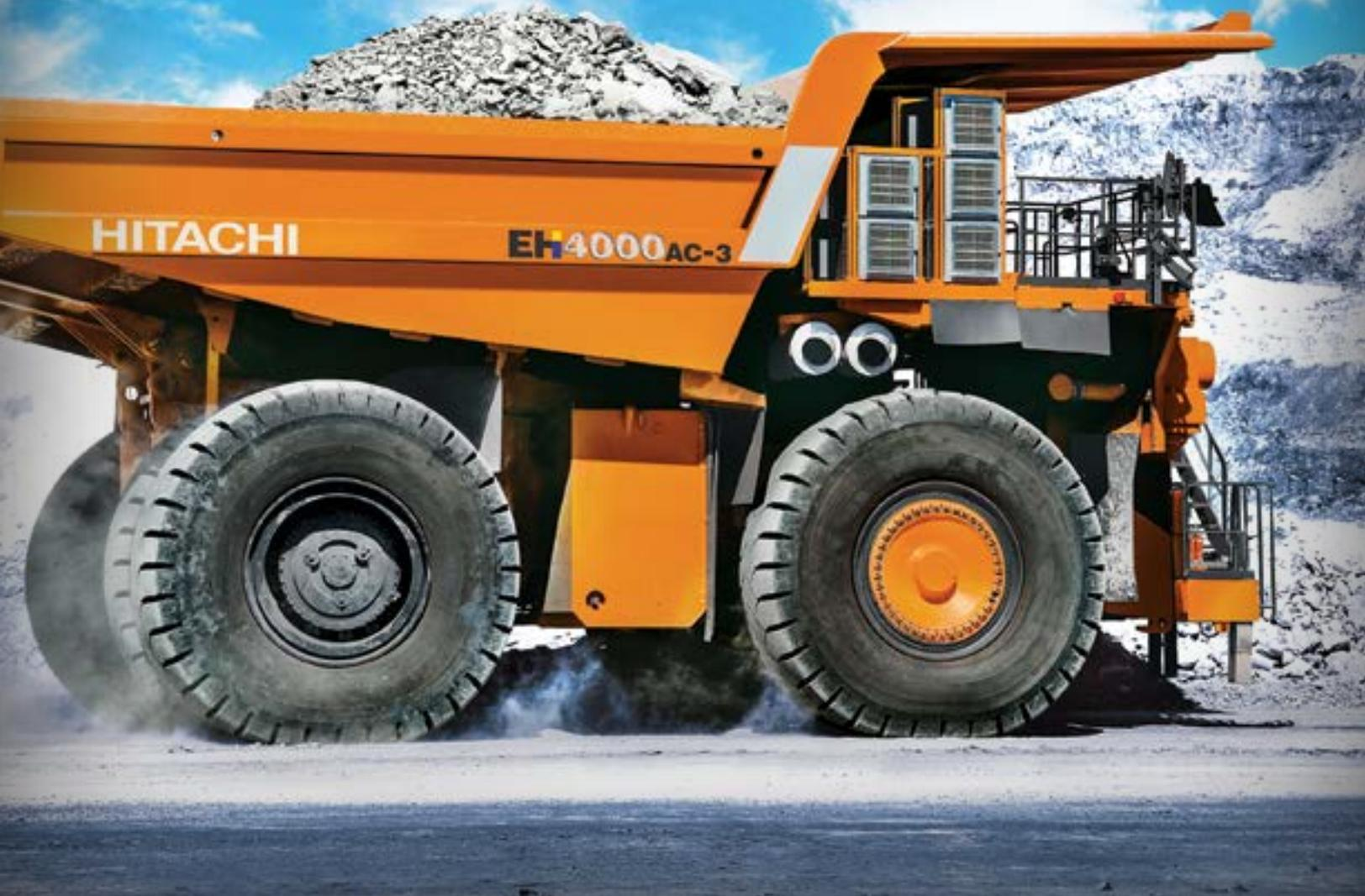
■ The box section design of the frame features one-piece top and bottom flanges that eliminate cross-member tie-in joints and provide a large, exposed center area for quick access to major components.
