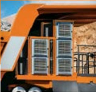
■ The AC-drive system has multiple controls that ensure trouble-free reliability and less maintenance. They include grid dry motor control that keeps the grid system dry in cold or wet conditions. A blower control cools the alternator and wheel motors in hot conditions.
