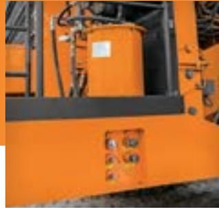
■ Hitachi trucks feature a fast-fill system station. This station, located on the left side of the radiator, gives you direct access at ground level for fast filling/topping off of lubricants, grease, hydraulic oil and engine oil. Our auto-lube system provides consistent lubrication to required areas on the truck reducing maintenance downtime. (Couplers are optional.)
