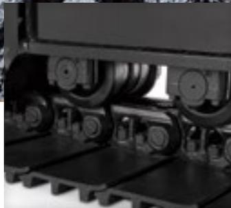
■ With large idlers, rollers and struted track links, the sealed and lubricated undercarriage is built for the long haul.
