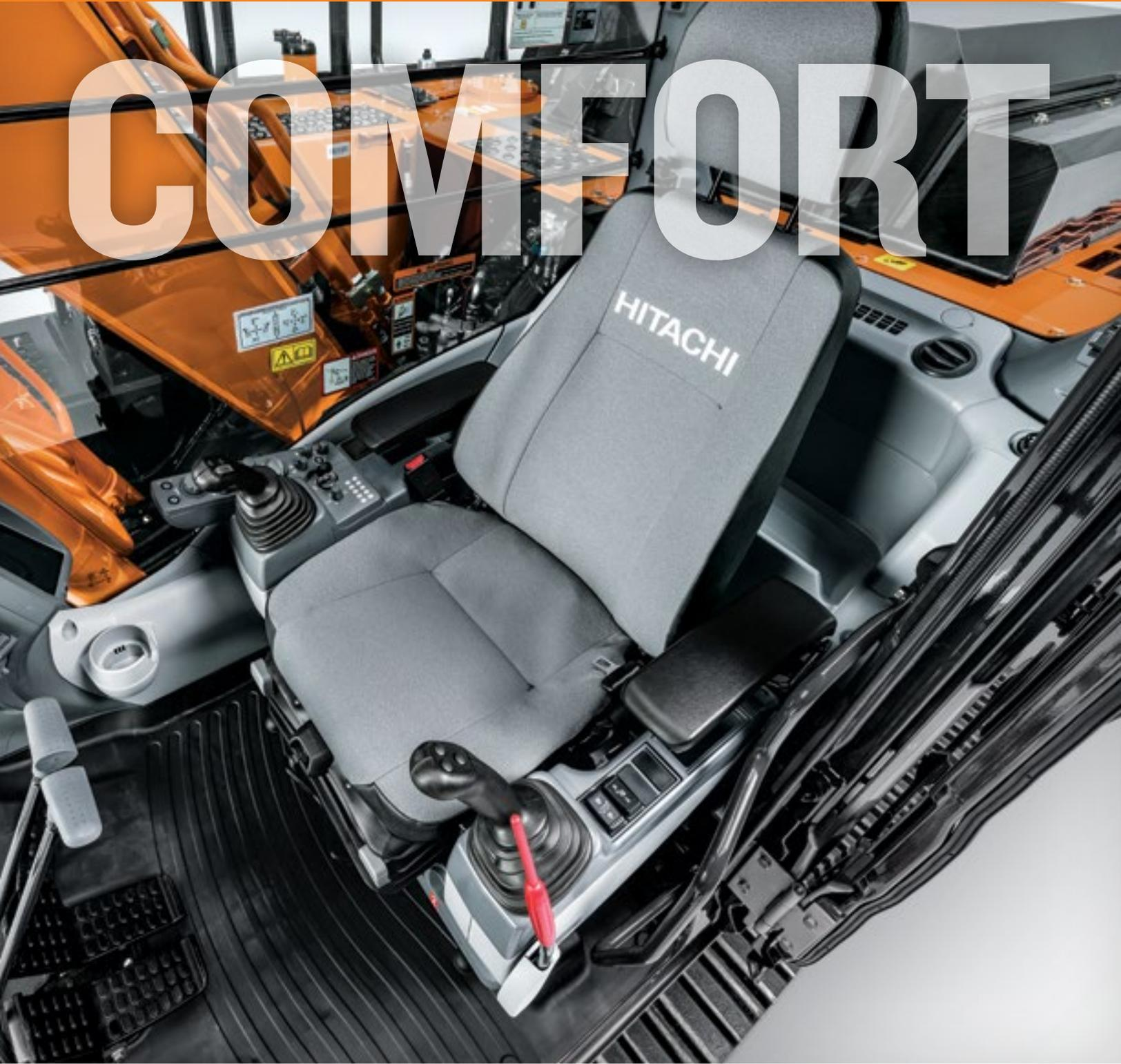
■ Automatic, high-velocity bi-level climate-control system with automotive-style adjustable louvers helps keep the glass clear, the cab comfortable and the operator productive.
