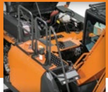
■ Upperstructure handrails provide added safety when servicing the engine compartment, and a larger hood gives you better engine accessibility.
