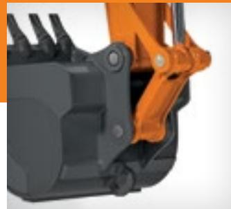
■ Tungsten-carbide-coated surfaces protect the critical bucket-to-arm joint.
