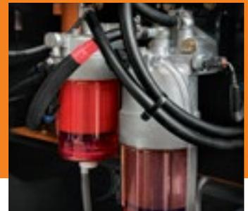
■ Engine oil, fuel and hydraulic pilot oil filters are all located on the same side at ground level for easy servicing.
