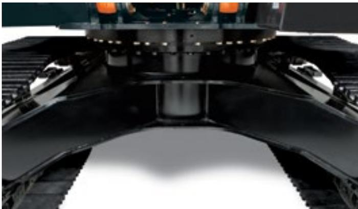
■ Thick-plate single-sheet mainframe, box-section track frames and industry-exclusive double-seal swing bearing deliver rock-solid durability.
