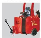
Low rear lift off or roll off for fast changeovers. Good access for battery topping. No motors underneath.
