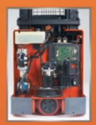
**Power unit tractor cover** is easily removed to provide access to major components. reducing service time during inspection and maintenance.
