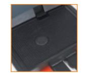
Low-effort. flush-mounted brake pedal allows increased freedom of movemen for greater operator comfort.
