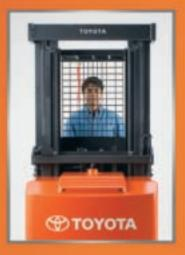
Wide-view mast with nested mast channels and side-mounted cylinders provide excellent visibility for improved pick rates.
