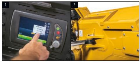
$Grade\text{-}control\ system\ includes\ Topcon\ 3D\text{-}MC^2\ components.$
